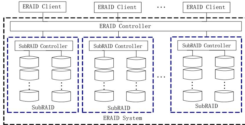
**Fig. 1.** Diagram of ERAID system architecture
