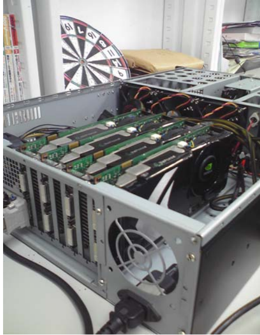
Figure 4: a 3U Compute Node with 4 Nvidia 8800GTS cards.
