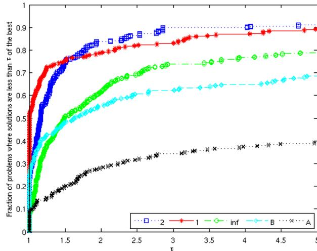
**Fig. 1.** Performance profiles for the condition number estimates for 245 matrices. A marks the condition number estimate of the original matrix; B marks that of Bunch’s algorithm [2]; inf, 1, and 2 mark that of the parallel scaling algorithm with  $\infty$ -, 1-, and 2-norms (with at most 25 iterations). At, for example  $\tau = 3$ , the curves from top to bottom correspond to the labels given in the legend from left to right.
