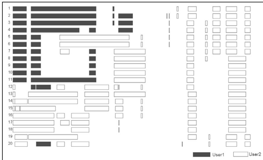
Fig. 5. Mapping of tasks to computer nodes with the global management; node number in the vertical axis and time in the horizontal axis
