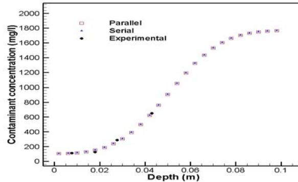
Fig. 2. Concentration profiles by using the serial and parallel codes.
