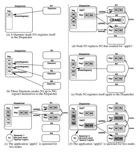
Fig. 2. The registering and spawning processes in JaceV.
